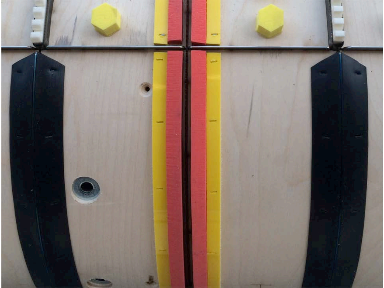
Container Graphics' LinerGuard™ shown with Surface Restraints (yellow) and used with Bundle Breaker Rule
